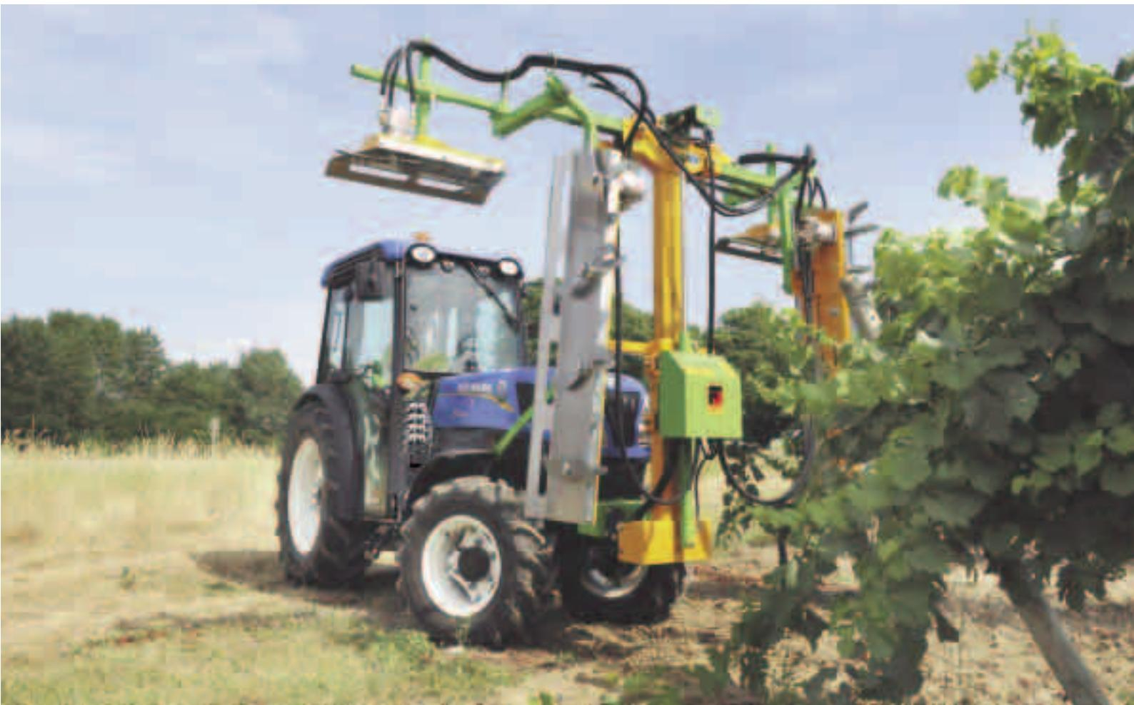
The modular build of T4F/N/V tractors enables New Holland to offer a broad range of specifications that exactly matches your specialised needs. T4 F/N/V models feature Megaflow™ High Volume, High Capacity Pumps, delivering an outstanding 63.8 LPM. All models benefit from a dedicated 35.6 Lpm steering pump. Regardless of engine speed or hydraulic load, full power to the steering circuit is maintained.
