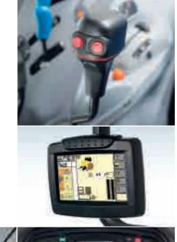
Control up to two mid-mount remotes with the integrated joystick which can be operated from the driver's seat for heightened comfort and productivity. The joystick has been ideally positioned on the Command Arc for intuitive operation.
