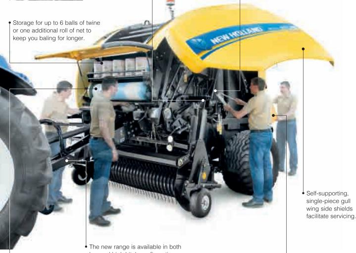
Optional storage for an additional four balls of twine. The new range is available in both low and high hitch configurations to suit both customer and market requirements.
